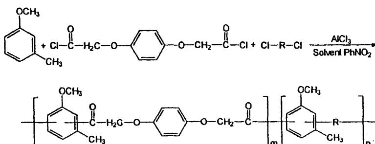
For resin no. 3 :  $\text{R} = -\text{CH}_2\text{CH}_2-$ For resin no. 4 :  $\text{R} = -\text{CH}_2-$
